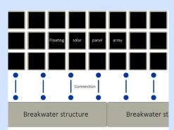
Geometric boundaries and material properties are also significant considerations in our project. We investigate the impact of FB geometry on wave attenuation and determine harmful wave spectrums for the FPV system, establishing necessary attenuation levels. Furthermore, we explore using ultra-high-performance fibre-reinforced concrete (UHPFRC) as an innovative material to enhance strength while reducing overall weight compared to traditional materials.
