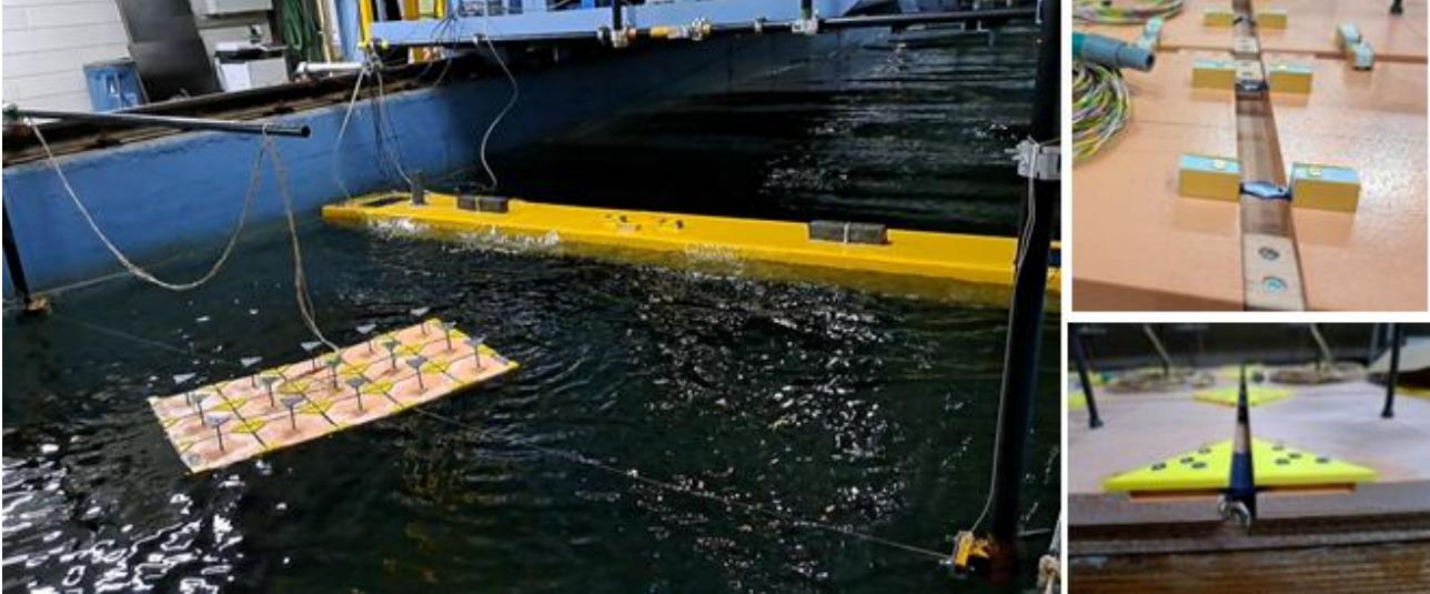
Figure 3: Basin model tests (left), initial hinge design lacking compressive stiffness (top right) and improved hinge design (bottom right).
